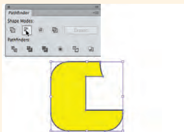
Minus Front removes overlapping areas from the backmost shape in the selection.
